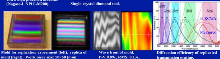
Mold for replication experiment (left), replica of mold (right). Work piece size: 50x50 [mm].
