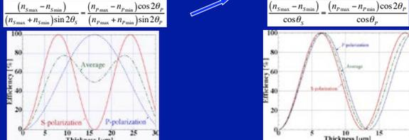
Polarized diffraction efficiencies of Dicon's VPH grating (Polarizer) calculated by Kogelnik method.
