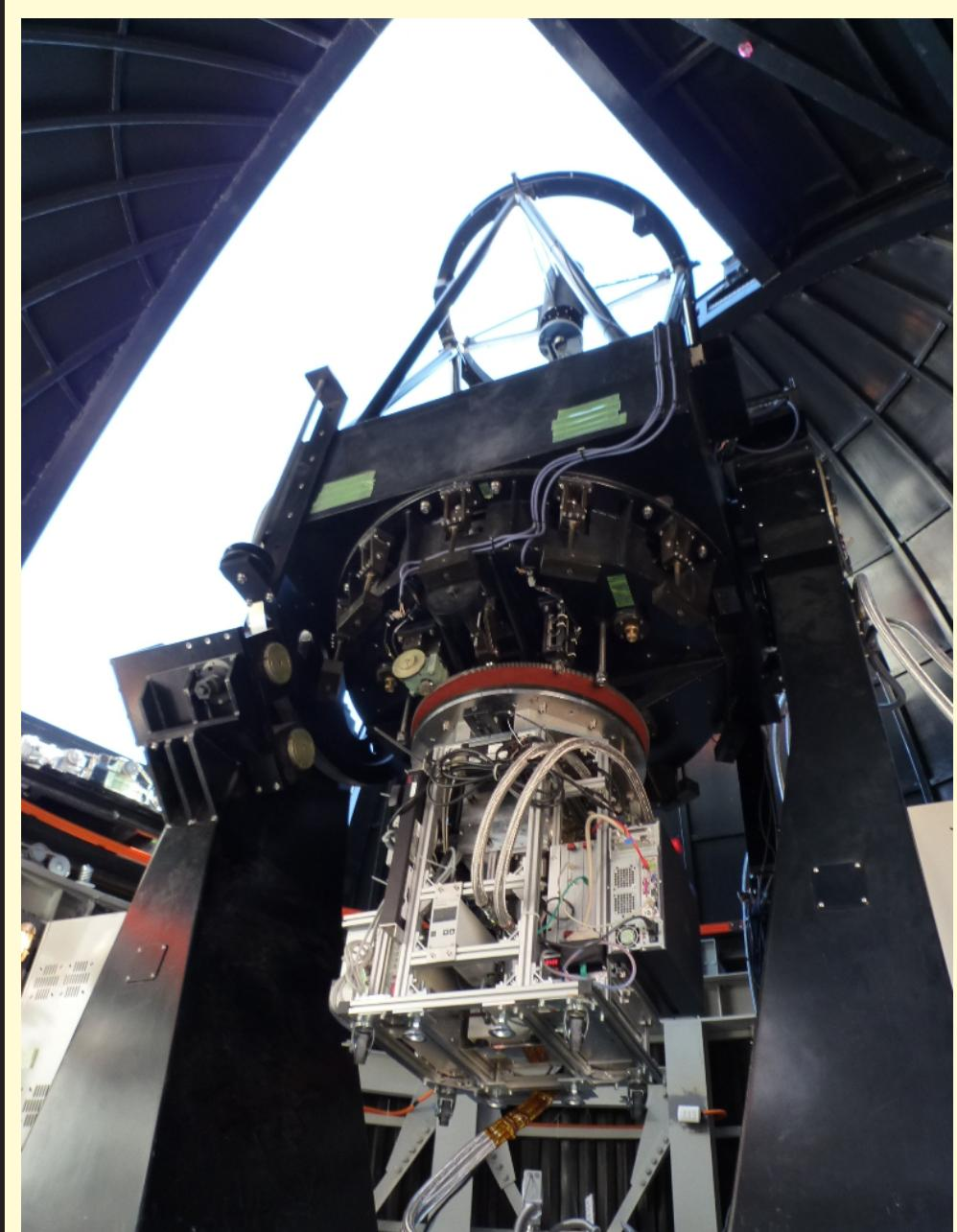
FIG.1 ANIR mounted on the Cassegrain focus of miniTAO telescope
