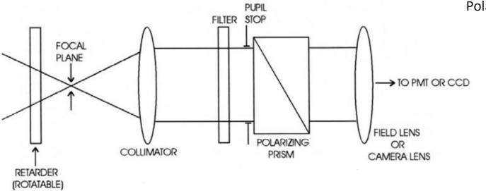
Polarizer: A specific linear polarization can only pass Rotator: Change the angle of polarization Retarder: Make phase shift in the beam
