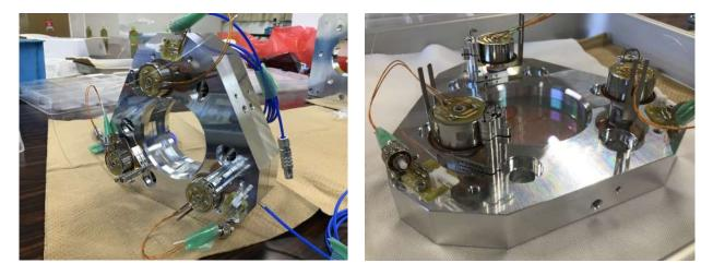
Figure 5. Aluminum housing with each component mounted.
