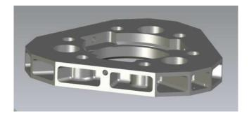
Figure 8. This model was designed to reduce weight while maintaining strength. A prototype made with a 3D printer has successfully reduced weight by approximately 37% compared to the current model.
