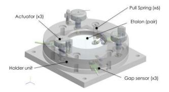
Figure 3. Conceptual design of Fabry-Perot module and layout of each component. This geometry allows the etalon to be freely displaced in three dimensions while at the same time allowing the gap to be measured.
