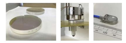
Figure 4. (left) Etalon (center) Piezo actuator (right) Capacitance gap sensor.
