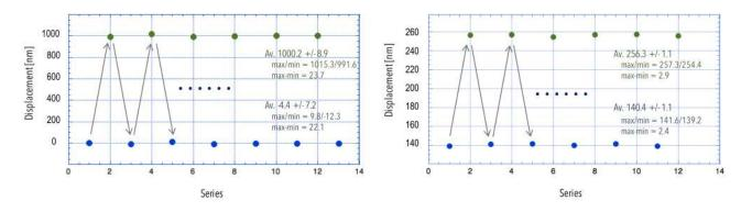
Figure 7. Results of multiple repetitive test (left : long range, right : short range). Uncertainty (stdv) before and after movement are about (1) 10 nm and (2) 1 nm respectively. Time drift was corrected for each results.
