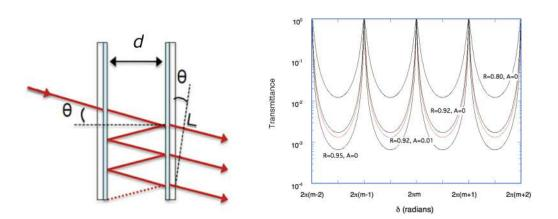
Figure 1. (left) Principle of Fabry-Perot interferometory. (right) Transmittance profile of Fabry-Perot interferometer (Airy function).
