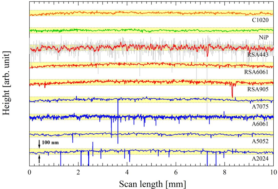
Fig. 6.6 Shape of surface finished mirrors. Plotted curve corresponds to path-A in Fig. 6.3b. The vertical axis gives an offset to improve visibility. Each yellow-filled areas indicates the range of P-V 100 nm corresponding to our requirements. The gray curve for RSA443 represents raw data, and the red curve drawn on it is obtained from simple moving average processing.
