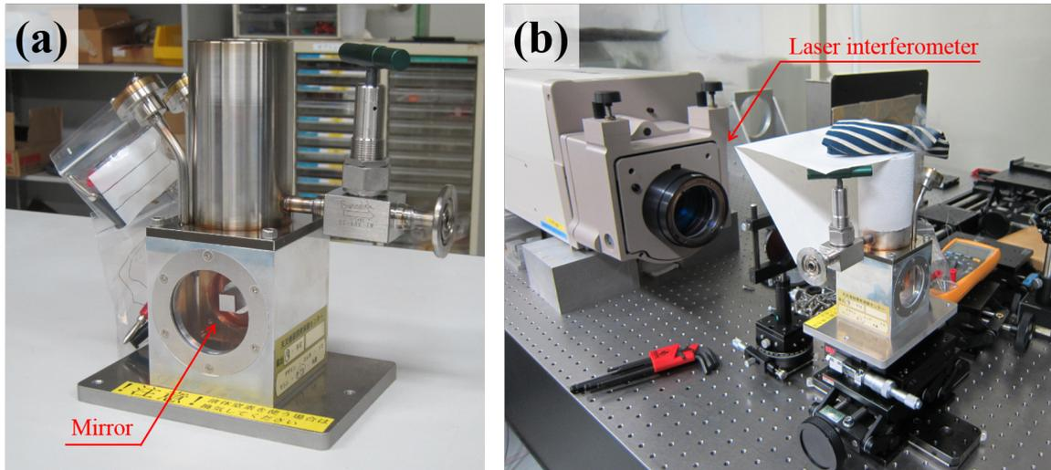
Fig. 6.7 (a) A cryo-dewar which cools mirror to LN2 temperature ( $\sim 80$  K). It has an optical window and a mirror mount made of oxygen-free copper. (b) The setup of measurement, with the laser interferometer and the dewar at the optical laboratory of Mitaka, NAOJ.
