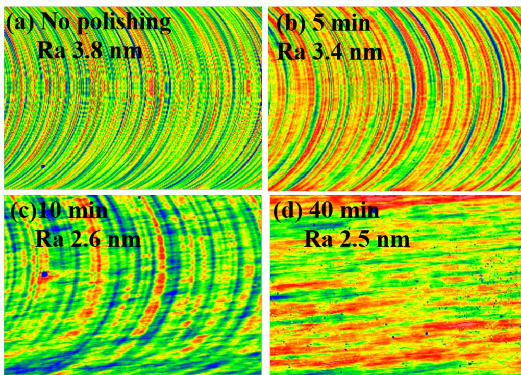
Fig. B.1 Results of post-process polishing by hand. The size of the measurement region is  $702 \mu\text{m} \times 526 \mu\text{m}$ . The time of the polishing changes with (a)–(d).
