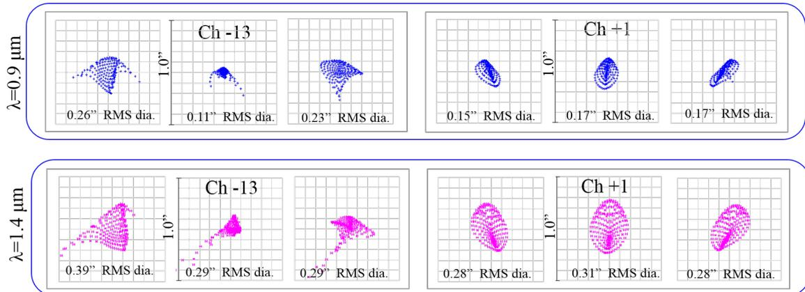
Fig. 4.10 Spot diagram at the detector of the blue arm of SWIMS. One side of the outer rectangle represents  $1.''0$  ( $= 10$  pixels) The upper row and the lower row show spots at  $0.9 \mu\text{m}$  and  $1.4 \mu\text{m}$ , respectively.
