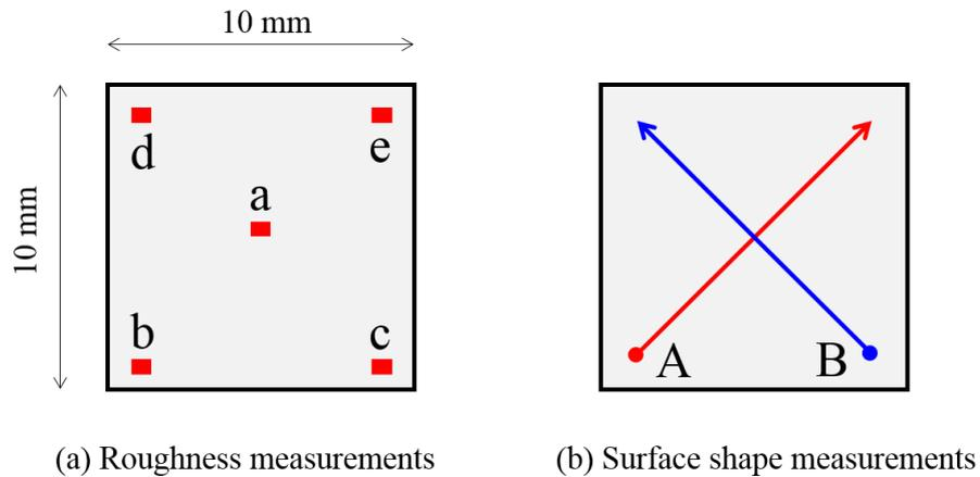
Fig. 6.3 Configuration of surface measurements. (a) Roughness is measured at five region (a–e) with size of  $702 \mu\text{m} \times 526 \mu\text{m}$ . (b) Surface shape is measured by scanning diagonally (path-A and -B) with length of 10 mm.
