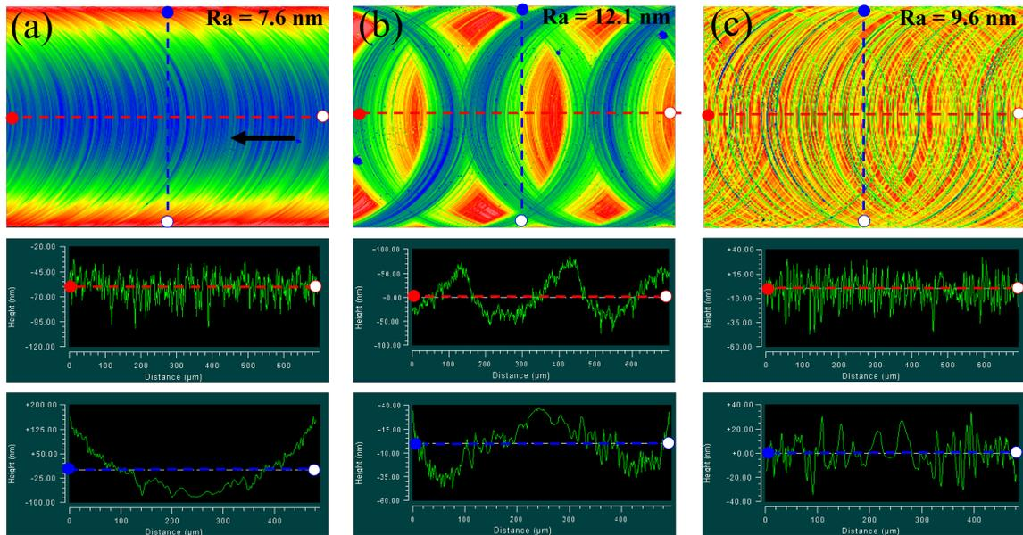
Fig. 5.7 Surface roughness after end milling. (a), (b), and (c) correspond to condition A, B, and C described in Table 5.3, respectively. Top panels represents surface profile for each conditions. Middle and bottom panels show the sectional shape of the region drawn with blue and red dashed lines in the top panel, respectively. Black arrow in the upper left panel indicates processing directions.
