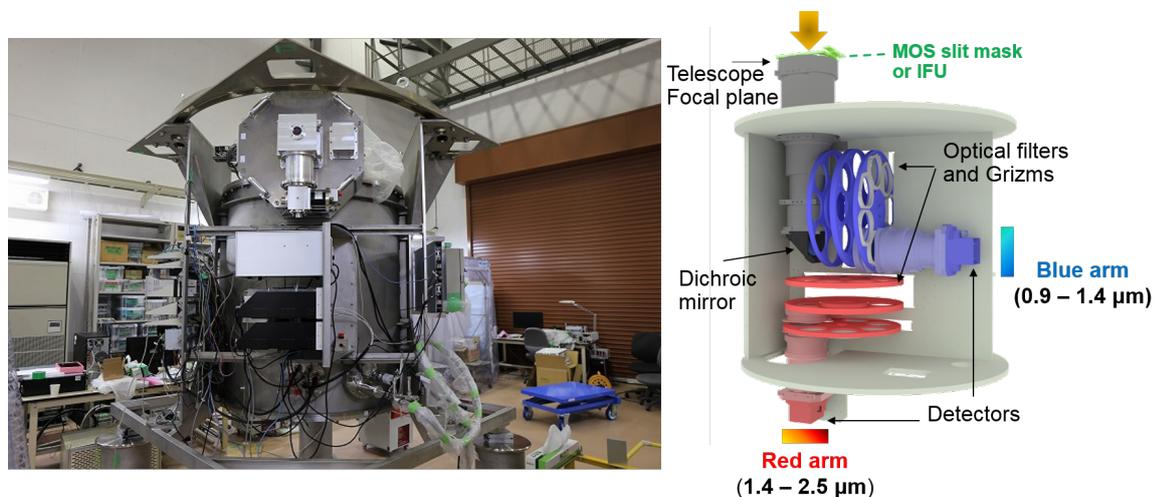
Fig. 3.1 *left*: Assembled structure of SWIMS components, which cryostat and the slit mask exchanger for MOS and IFS observation (see also Fig. 3.2). *right*: Layout of SWIMS optics with its optomechanics optimized for the Subaru telescope. The mask exchanger is not drawn in this figure. The incident light from the telescope is divided into the blue arm (0.9–1.4 μm) and the red arm (1.4–2.5 μm) with the dichroic mirror. Each camera lens is optimized for each wavelength band.
