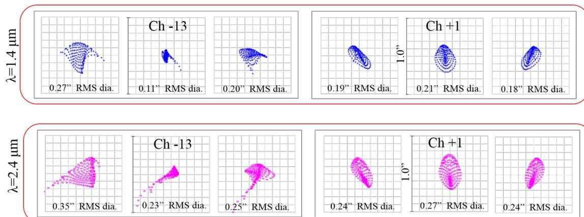
Fig. 4.11 Spot diagram at the detector of the red arm of SWIMS. One side of the outer rectangle represents  $1.''0$  ( $= 10$  pixels) The upper row and the lower row show spots at  $1.4\mu\text{m}$  and  $2.4\mu\text{m}$ , respectively.
