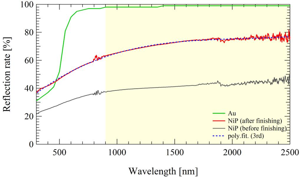
Fig. 4.15 The measured reflection of NiP surface mirror. The yellow filled area shows the wavelength range of SWIMS. The ripples seen at  $\sim 800$  nm and  $\sim 1800$  nm are caused by the exchange of detectors. The curve of finished workpiece (2nm rms) is fitted with a cubic function and results is as follows.  $R = 15.01 + 0.082544 \lambda - 3.8578 \times 10^{-5} \lambda^2 + 6.1892 \times 10^{-9} \lambda^3$ .
