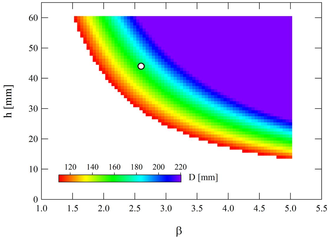
Fig. 4.3 The paraxial parameters which gives the solutions of  $F(x) = 0$  with  $0 < x < h$ . The search ranges of each parameter are  $D = 110\text{--}220$  mm,  $h = 0\text{--}60$  mm, and  $\beta = 0.0\text{--}5.0$ , respectively. The white circle indicate the set of  $(D, h, \beta)$  we used for calculating the paraxial optical layout.
