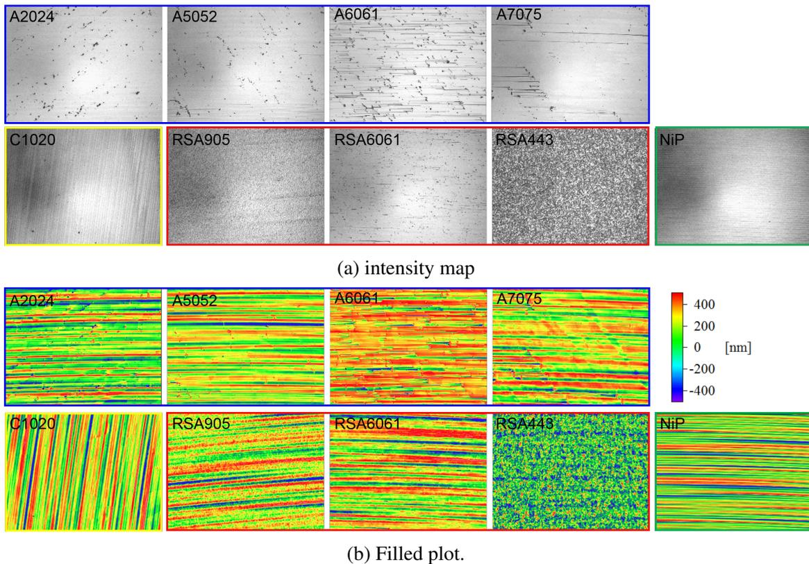
Fig. 6.4 Surface profile at the region “a” of each material with field-of-view of  $702 \mu\text{m} \times 526 \mu\text{m}$  (a) Intensity maps which are useful for distinguishing fine grains (e.g. black dot-like feature) on the surface (b) Filled plots which clearly show depth and direction of cutting marks. Each field of view is same as that of (a).
