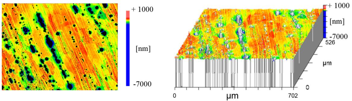
Fig. 6.10 Surface profile of NiP plating with a thickness of  $5\ \mu\text{m}$ . Many pores appear on the surface after diamond cutting. Some pores has a depth of  $7\ \mu\text{m}$ , and it reaches an aluminum substrate.
