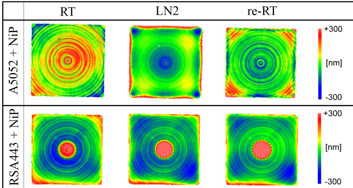
Fig. 6.8 Results of shape measurements. RT, LN2, and re-RT represent room temperature (300 K), liquid nitrogen temperature (77K), and room temperature after the thermal cycle (*i.e.* after elevating temperature). The top and bottom rows show the shape changes of A5052 and RSA443 with 100  $\mu\text{m}$  of NiP plating at each temperature. Spike noise is removed by performing sigma clipping at each temperatures.
