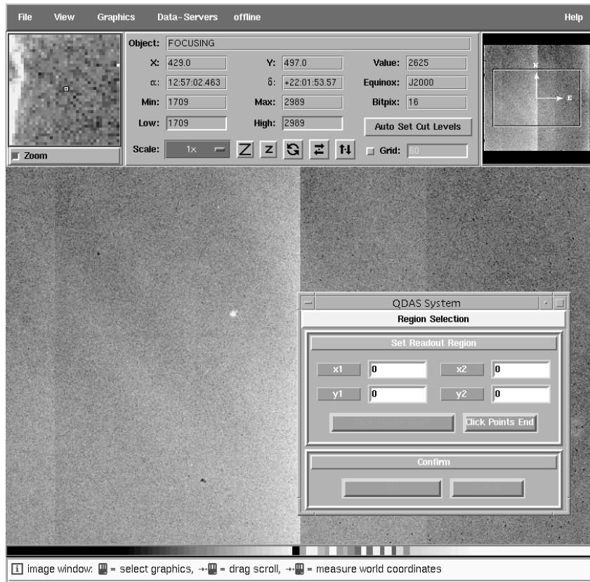
When finished, the plot of FWHM-Z relation and the best focus position are displayed in "QDAS plot" window as below.
