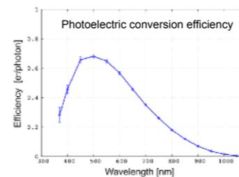
Figure 3. Response function of the Tomo-e camera.
