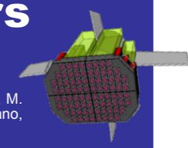
**Tomo-e Gozen** (Tomo-e) is a wide field optical camera equipped with 84 CMOS sensors for the Kiso 1.05 m f/3.1 Schmidt telescope operated by the University of Tokyo. Tomo-e is capable of taking optical images of **20 square degrees** consecutively in **2 fps**. A camera unit equipped with the 21 CMOS sensors have been completely developed in February, 2018 (Figure 1). In this poster, evaluations of the CMOS sensors and sensitivity estimation of Tomo-e are reported.
