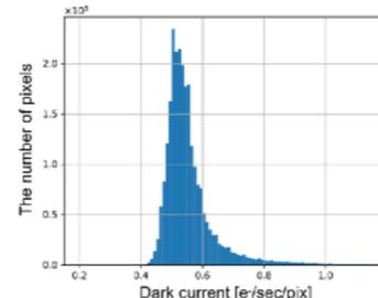
Figure 4. Distribution of the dark current at 290 K.
