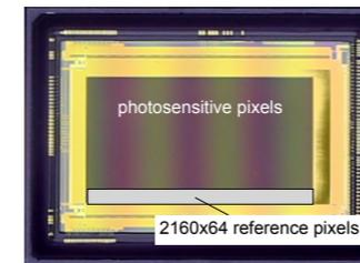
Figure 2. Canon 35MMFHDXM 35 mm CMOS sensor
