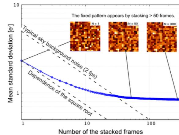
Figure 5. Noise reduction by stacking dark frames subtracted the self bias frame.
