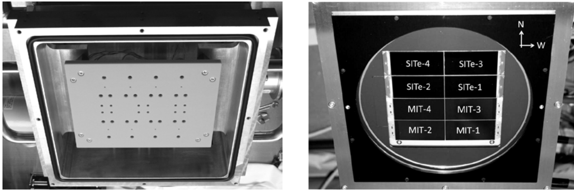
Figure 2. Left: AlN cold plate installed in the cryogenic dewar. The cold plate is supported by fiber reinforced plastics (FRP) plates at the four corners. Right: Top view of the cryogenic dewar with the CCDs and the flattener lens. The MIT and the SiTe CCDs are placed in the south and the north sides on the image area, respectively.
