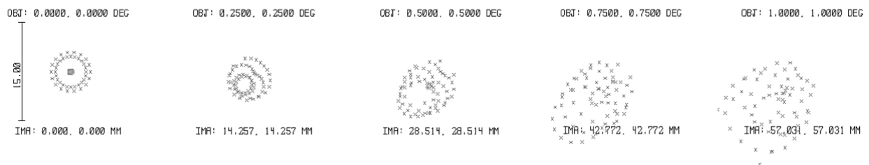
Figure 8. Spot diagrams for the KWFC mounted on the Kiso Schmidt telescope at 0.55 \mu\text{m} wavelength. The distances along the x- and y- axes of the image file from the optical center are indicated at the top of each image in degrees. The physical distances are also indicated at the bottom of each image in mm. Solid bar indicates a physical size of the CCD pixel in microns. Most energy of a PSF is focused inside a CCD pixel with a size of 15 \mu\text{m} .
