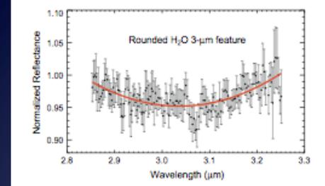
Fig. 6. Isolated rounded 3-μm feature in the spectrum of 361 Bononia. The best fit for this feature is a second order polynomial across the 2.85–3.25-μm region (in red). (For interpretation of the references to color in this figure legend, the reader is referred to the web version of this article.)
