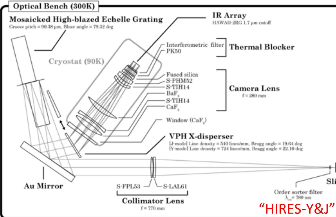
Figure 2. Optical layout of WIDE-mode (top) and Hires-Y and J modes (bottom) of WINERED. The optical elements are located on the optical bench with the room temperature, except for the camera lens and infrared array that are installed under the cryogenic condition with  $T = 90 \text{ K}$  and  $77 \text{ K}$ , respectively. See text for more details.
