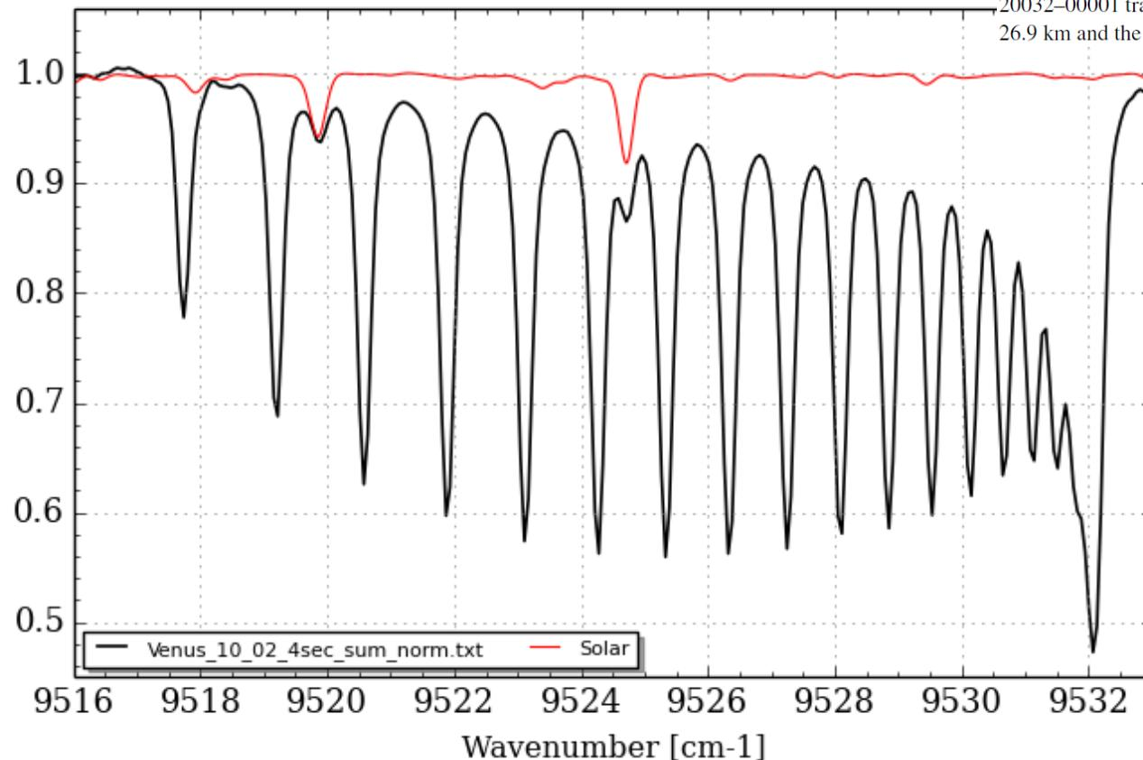
FIG. 1. Section of the ICLAS spectrum in the region of the  $R$  branch of the 20032–00001 transition of  $^{12}\text{C}^{16}\text{O}_2$ . The equivalent absorption path length was 26.9 km and the sample pressure was 32.7 Torr (43 hPa).
