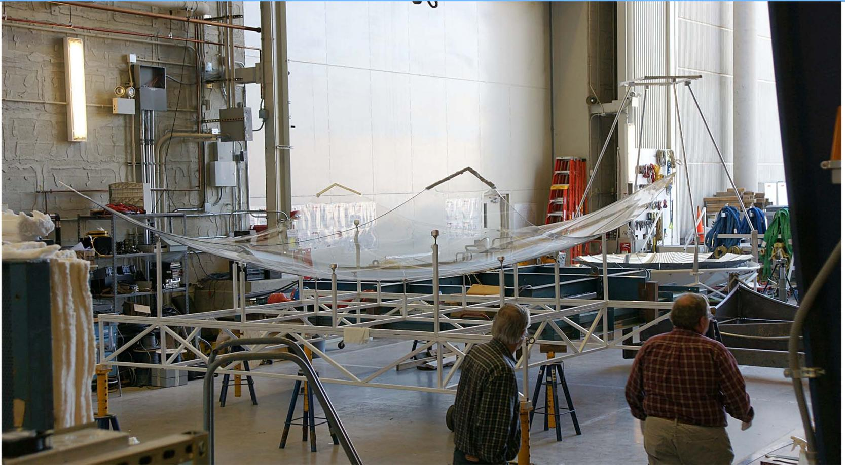
First slumped 3m x 3m reflector. Process still under development. Also need efficient means of backside coating with silver and applying protective covering. Individuals shown are Roger Angel and Materials Scientist, Blane Olbert.
