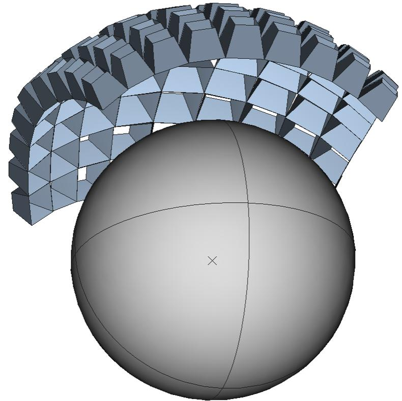
Image of 3 m square reflector feeds many cells, all with same flux. Note, the individual concentrator elements,
