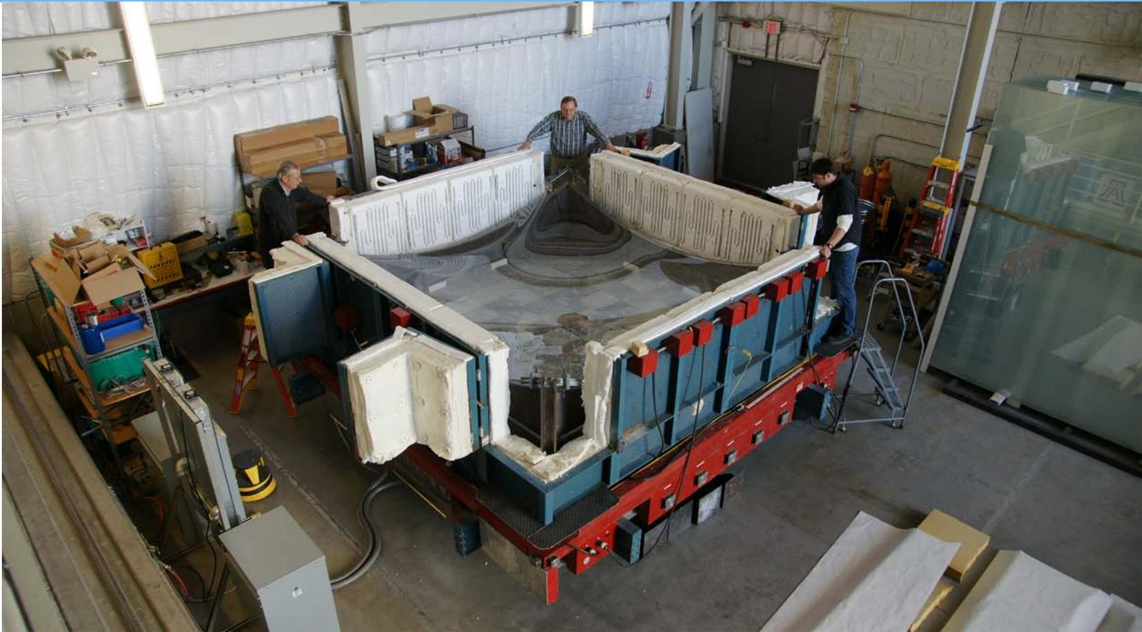
The prototype slumping furnace in the UA Mirror Lab. In production, the float glass sheets need to be slumped at same rate, 1 per 10 seconds, as they are produced. At that rate can build capacity of ~7.5 Gigawatts per year per float glass factory.
