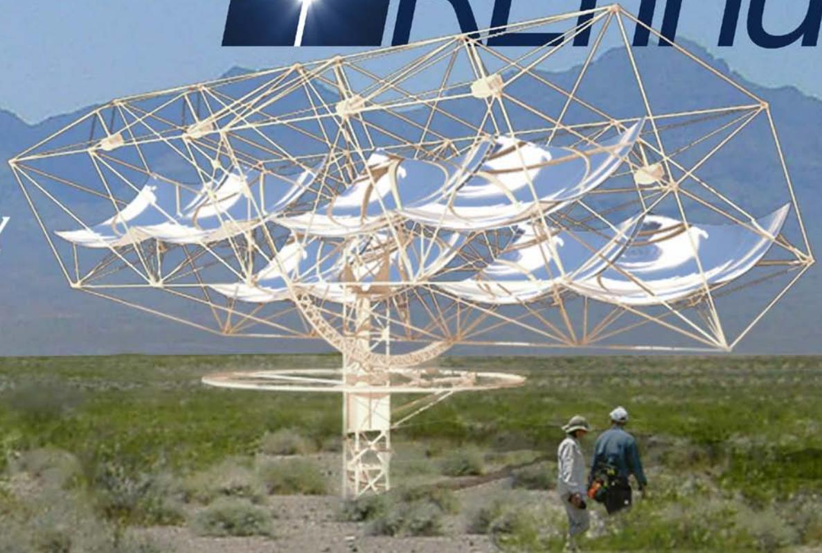
Advantages; Stiff: Low mass: Simple tracker mechanism: Minimal environmental impact: 8 float glass sheets: Low self-shadowing in array "farm"; Capacity 20KW
