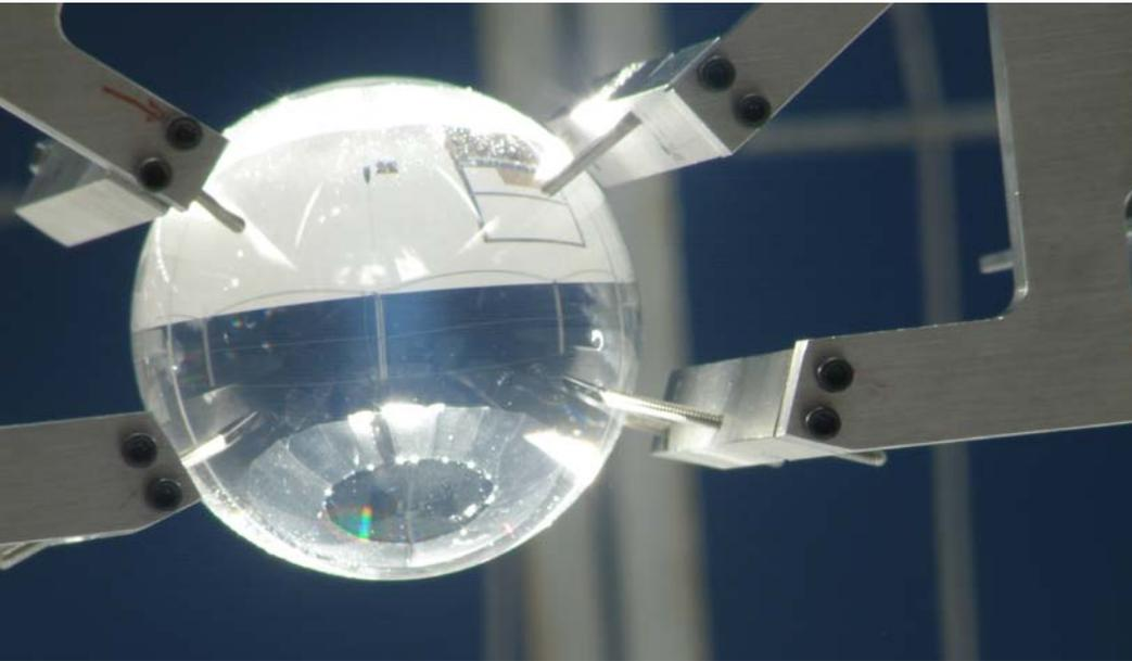
The sunlight from each dish is focused in the center of a sphere of pure fused silica - the blue glow is Rayleigh scattering
