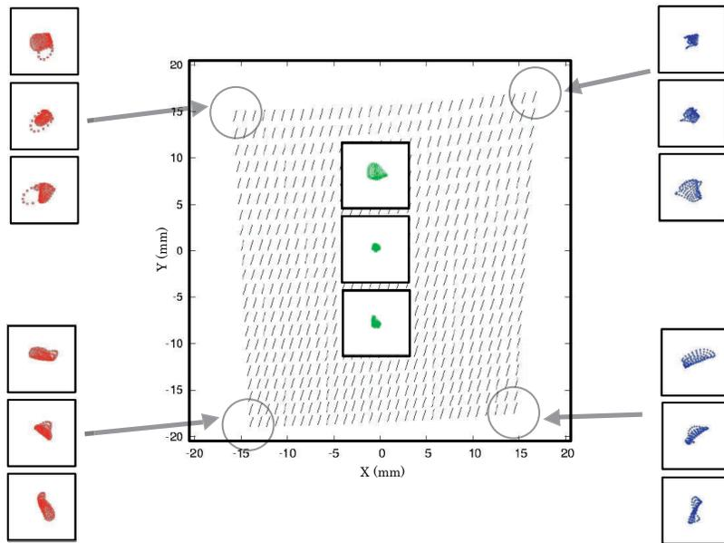
**Figure 4.** Echelle format and spot diagrams for the Y-mode. We obtained the spot diagrams at five detector positions, thereby at five wavelengths. The three boxes at each detector position show the spot diagrams at the upper edge, center, and lower edge of the slit, respectively. The boxes represent  $2 \times 2$  pixels.
