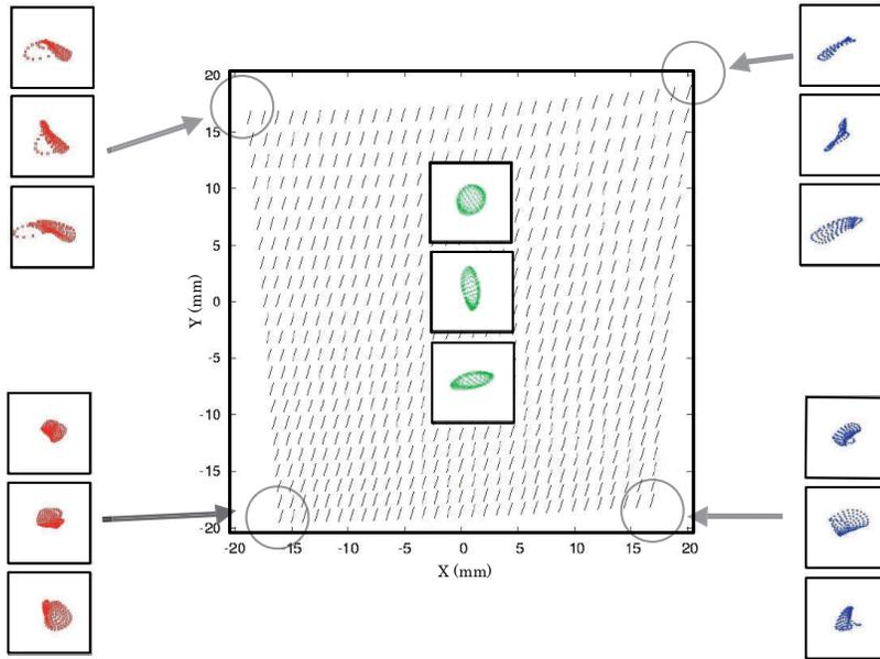
**Figure 5.** Echelle format and spot diagrams for the J-mode.
