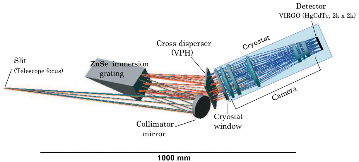
**Figure 1.** Optical layout of WINERED in the immersion grating mode. For the normal echelle mode, the immersion grating is replaced with a normal echelle.
