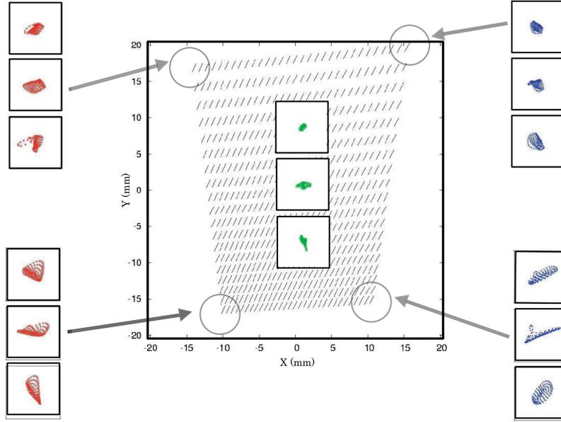
**Figure 6.** Echelle format and spot diagrams for N-mode.
