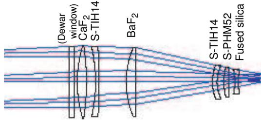
**Figure 3.** Optical layout of WINERED camera system. The leftmost flat of the figure shows a dewar window of CaF<sub>2</sub>.
