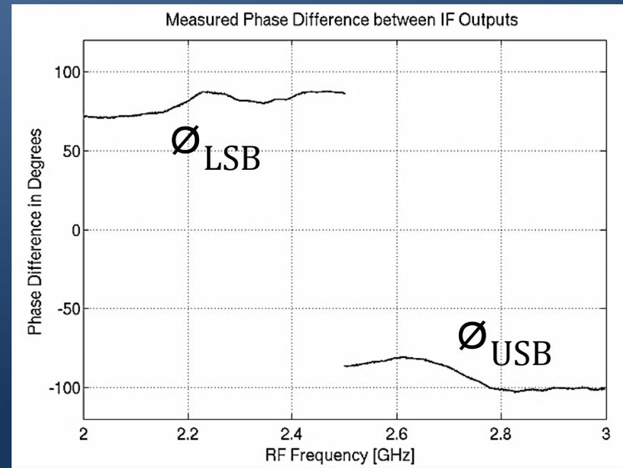
Measured USB and LSB amplitude ratio  $X$  (left) and phase imbalances  $\phi_{LSB/USB}$  (right).
