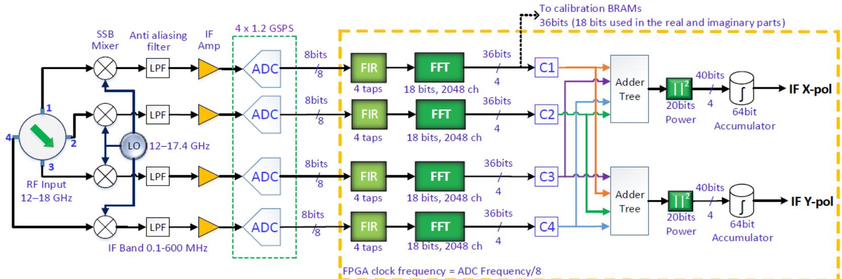
FPGA (Virtex-6) processing platform (ROACH II)
