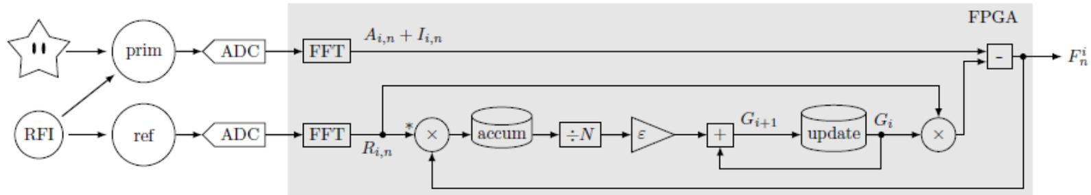
Figure 1: Schematic of the adaptive filter.
