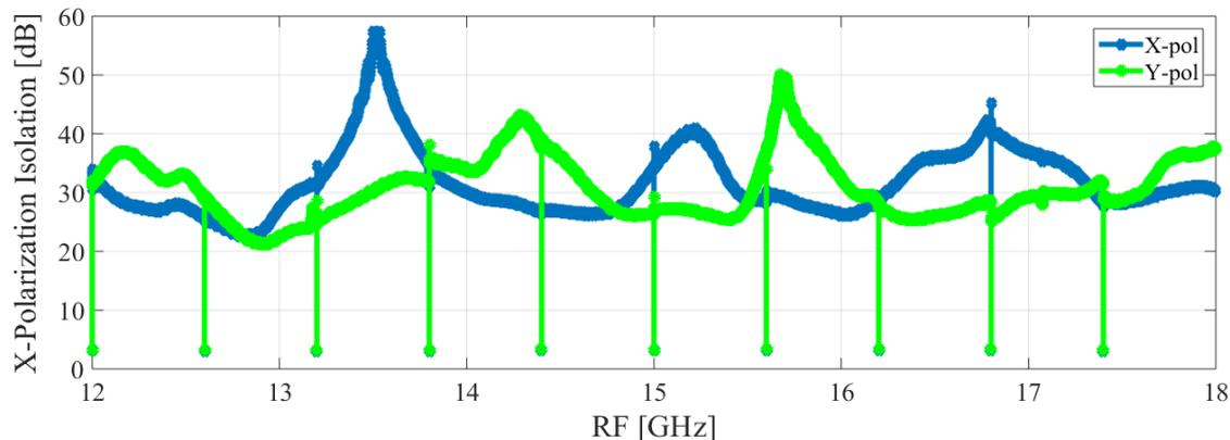
Calibrated Cross-Polarization Isolation. Ku-Band
