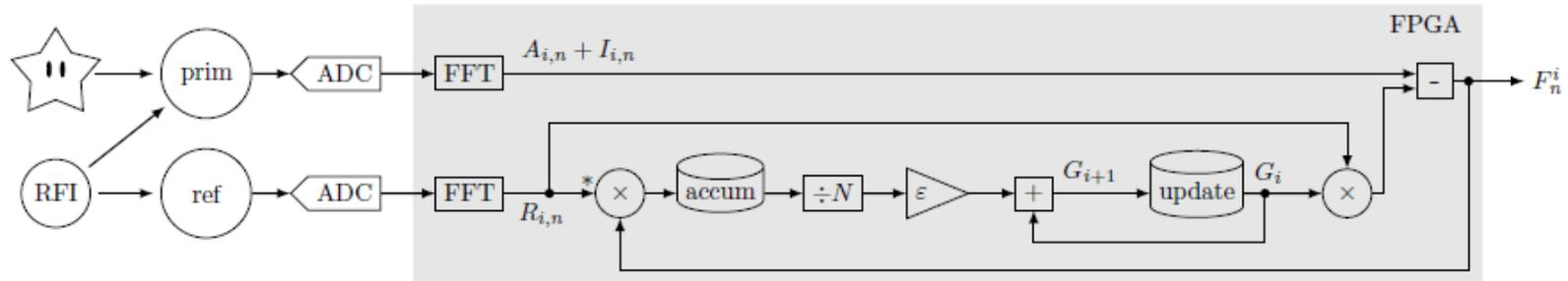
Figure 1: Schematic of the adaptive filter.
