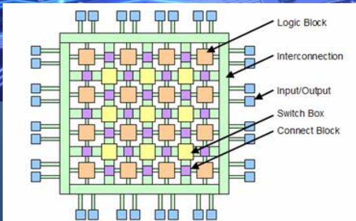
**FPGA fabric schematic**
