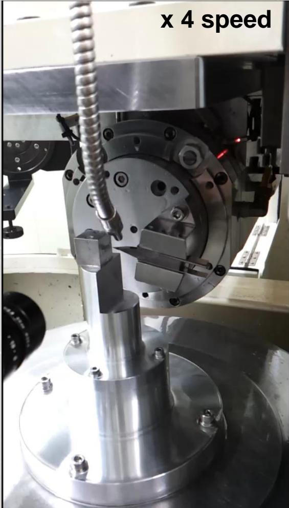
► Fabrication of slice mirror arrays
