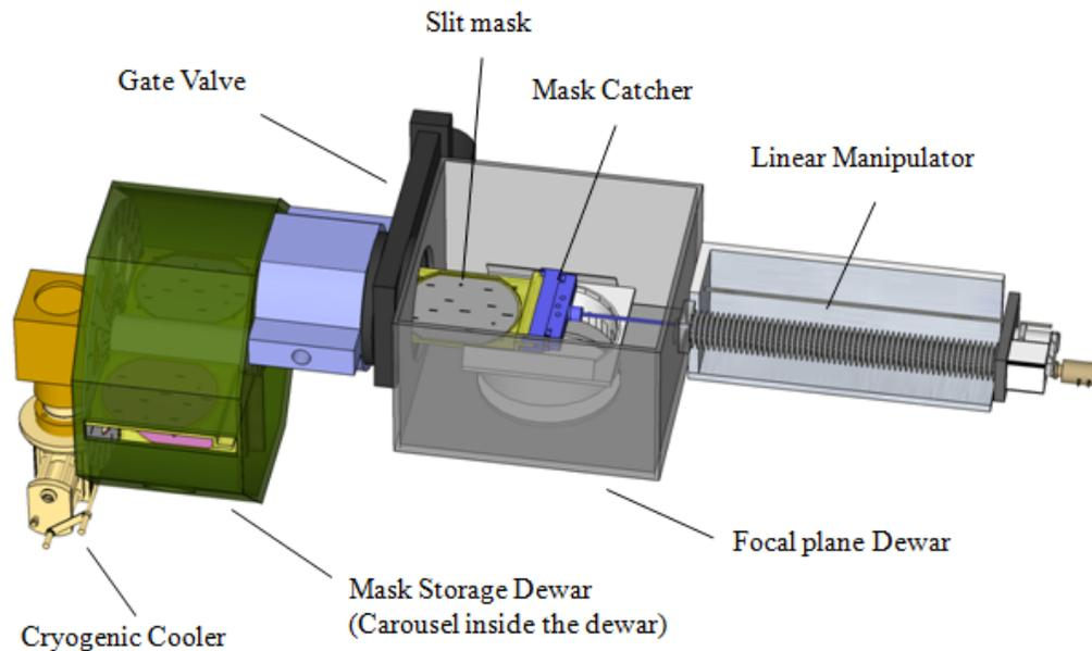
Figure 7. 3D schematic view of the MOS unit. The overall length of the unit is about 2400mm. The telescope focus is located in the focal plane dewar, where a slit mask is set.
