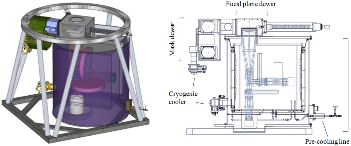
Figure 2. 3D (*left*) and 2D cross-sectional (*right*) schematic drawings of SWIMS. The interface and support structures for the Cassegrain focus of the Subaru Telescope are also shown in the *left* panel. Dimension and weight of SWIMS are approximately  $2 \times 2 \times 2 \text{ m}^3$  and 2 tons.
