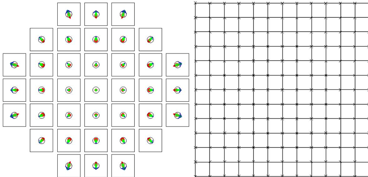
Figure 5. Similar to Figure 4, but for the *red* channel. For each diagram in the *left* panel, the red, blue, and green spots correspond to wavelengths of  $\lambda = 1.4, 1.8,$  and  $2.4 \mu\text{m}$ , respectively, and the circle represents the Airy disk at  $\lambda = 2.4 \mu\text{m}$ .
