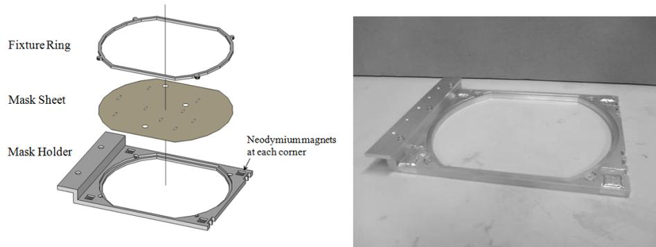
Figure 8. Schematic drawing of the slit mask (*left*) and a prototype for positioning tests using neodymium magnets (*right*). The mask sheet is made of aluminum sheet and its shape is a combination of a circle (210mm in diameter) and a rectangle (150mm  $\times$  210mm).
