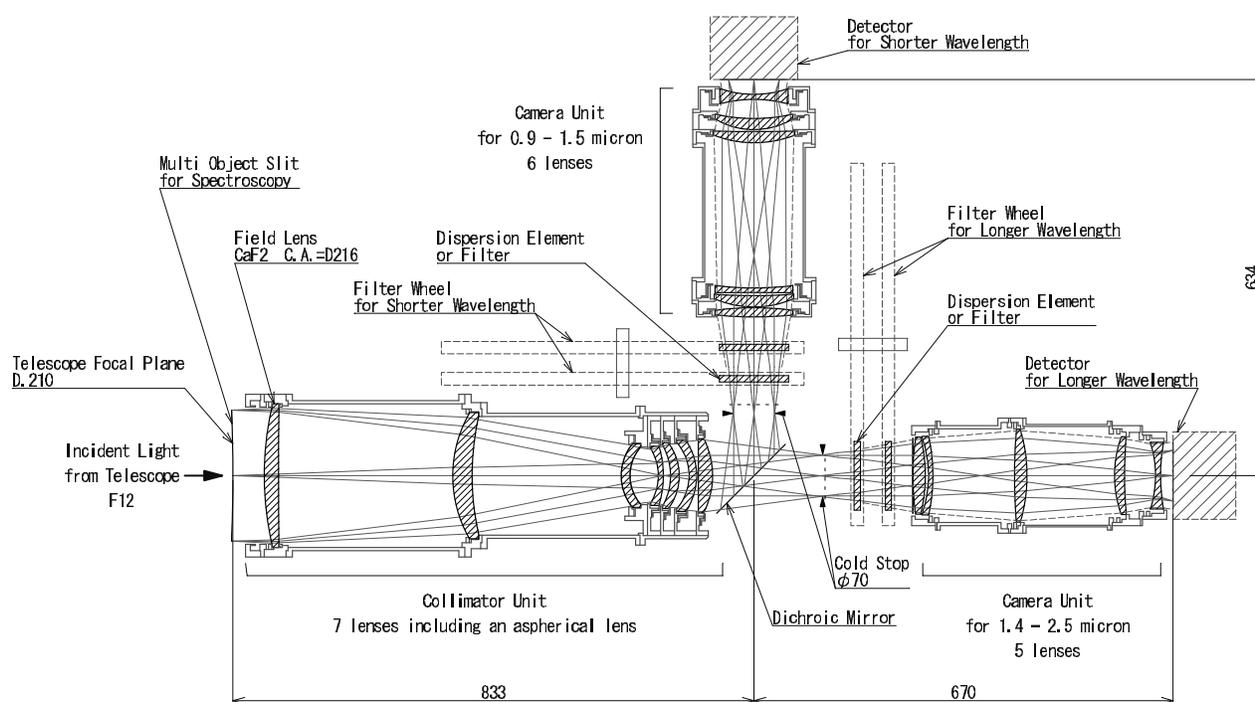
Figure 3. A schematic of the layout of the optics inside the SWIMS cryostat optimized for the Subaru Telescope.
