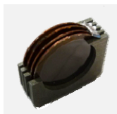
Figure 2. A Metal Mesh Filter. It is composed of four gold thin-films. The diameter of the films is about 10-mm, and the thickness of each film is 2-micron.
