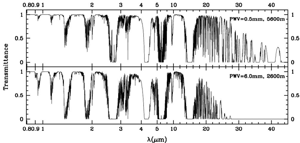
Figure 2. Comparison of atmospheric transmittances at 5,600m altitude (a model for Co. Chajnantor) and 2,600m (for Co. Paranal). At the summit of Co. Chajnantor, new atmospheric windows beyond the wavelength of 30 $\mu\text{m}$  appear, and the absorption bands in the near-infrared wavelength at 0.8 to 2.5 $\mu\text{m}$  almost disappear.
