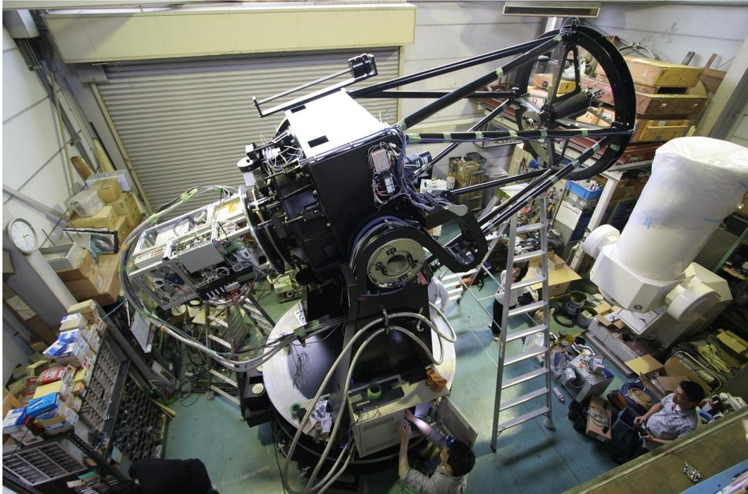
Figure 9. The 1.0m telescope pre-assembled in the factory at Kyoto, Japan. The MAX38 mid-infrared camera<sup>6</sup> is mounted on the Cassegrain focus.
