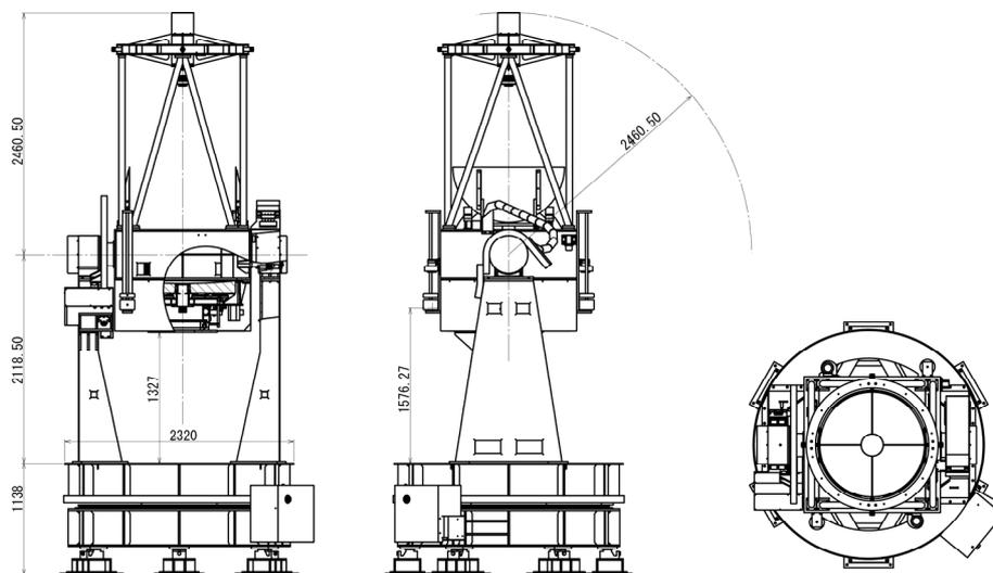
Figure 8. Schematics of the 1.0m telescope.
