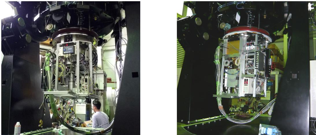
Figure 11. Photographs of the ANIR near-infrared camera (*left*) and the MAX38 mid-infrared camera (*right*) mounted on the Cassegrain focus of the 1.0m telescope.
