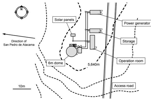
Figure 4. Layout of the summit facilities. The contour step is 1.0m. Up side is north. The telescope dome is placed on the southwest ridge of the summit, the windward side, to obtain better seeing.
