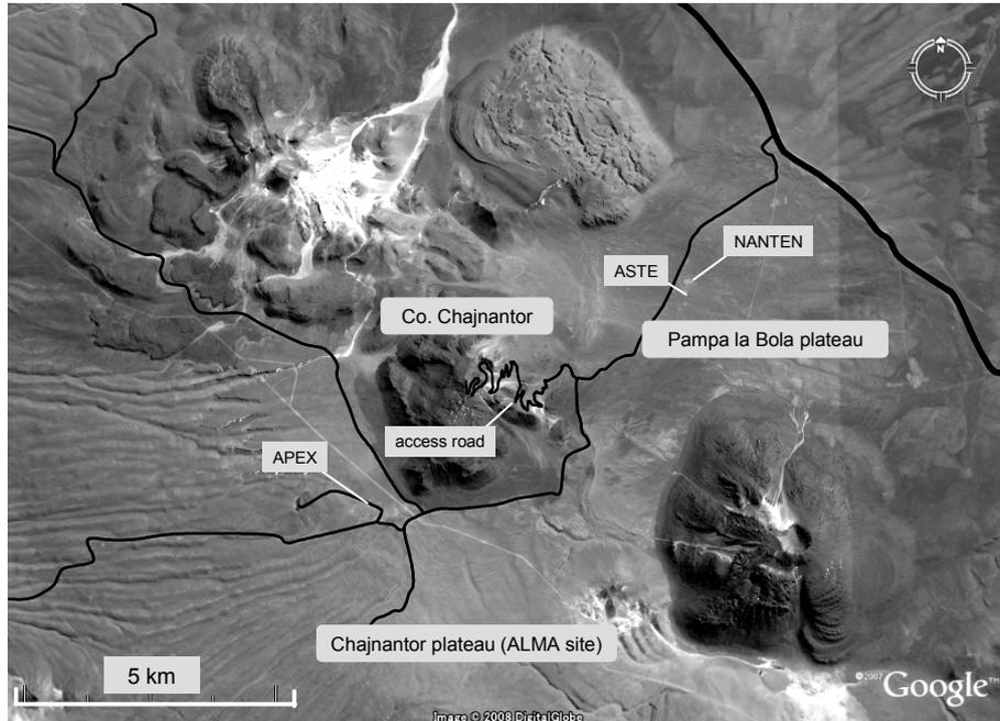
Figure 1. Map of the Chajnantor region. Up side is north. Co. Chajnantor lies between the Pampa La Bola plateau and the Chajnantor plateau. The access road to the summit is constructed on the east face, and the entrance is located at 5,150 m altitude on the opposite side of the ALMA site.
