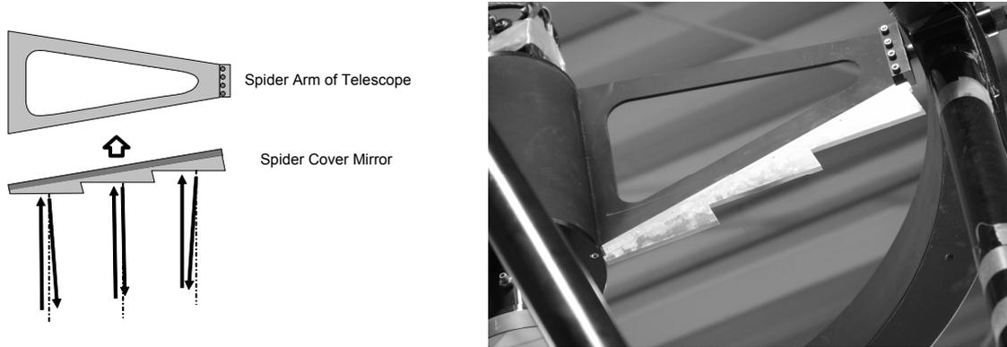
Figure 7. (left) Schematics of spider cover mirrors. All the mirrors are placed almost parallel to the primary mirror, but practically the cover mirrors near the secondary mirror are pointed slightly (1deg) outside and the mirrors near the top-ring slightly inside to reduce confusion of the emissions from the Cassegrain hole and the outside of the primary mirror, respectively. (right) Photograph of the spider cover mirrors installed at the spider arms.
