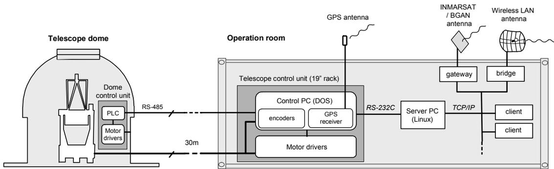
Figure 10. Diagram of control system for the 1.0m telescope. The 1.0m telescope and the 6.0m dome are managed with a DOS based control PC installed in the operation room. Users control the telescope and the dome via a Linux based server PC. The summit network is linked with the base support facility at San Pedro de Atacama by a wireless LAN bridge and a satellite communication.
