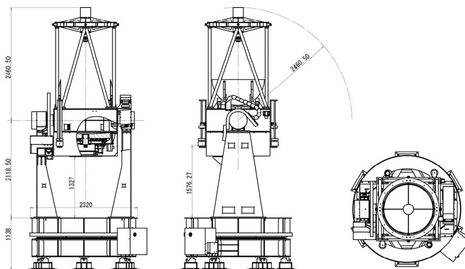
Figure 8. Schematics of the 1.0m telescope.
