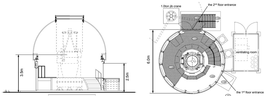
Figure 5. Schematics of the 6.0-m dome. (left) Cross-sectional elevation view from the first floor entrance. (right) Cross-sectional plane view. Up side is north. The 6m dome and the summit facilities are constructed by Kokusai Kogyo Co. Ltd and Nishimura Co., Ltd.
