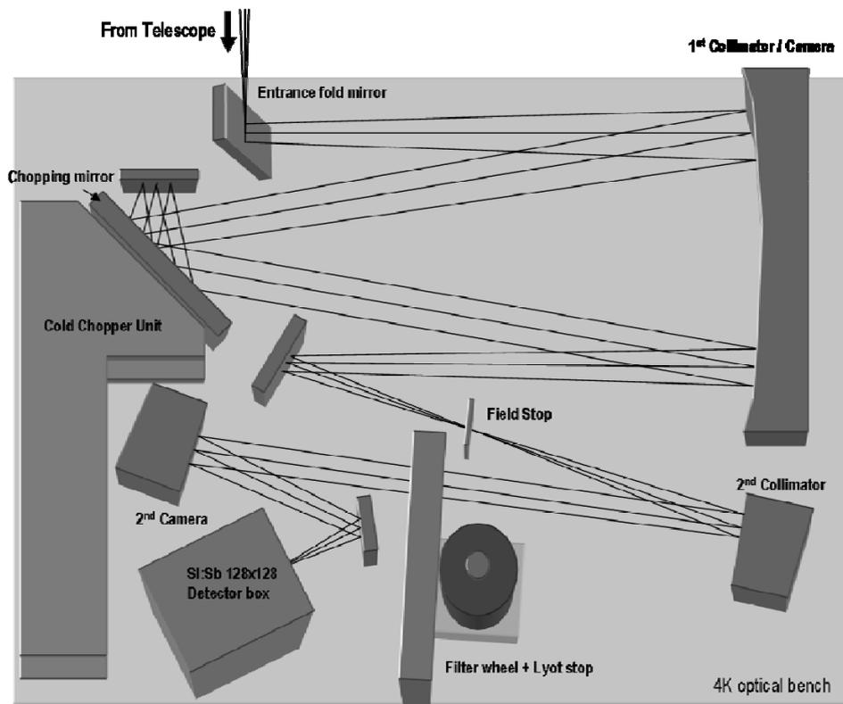
Fig. 2. Schematic drawing of the MAX38 optics. All components are mounted on the optical bench and cooled below 8K.
