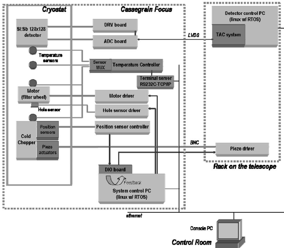
Fig. 3 Block diagram of the MAX38 control system. Components in the dotted box labeled “Cassegrain Focus” are mounted in the instrument carry and attached at the Cassegrain focus of the telescope. The detector control PC and the piezo driver are put in the computer rack attached on the telescope. All systems can be operated from console computer(s) via Ethernet.
