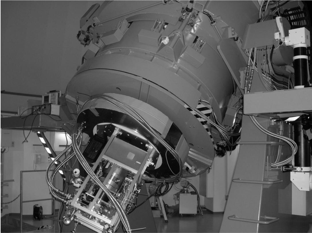
Fig. 4 The MAX38 mounted on the Kanata 1.5-m telescope at the Higashi Hiroshima Observatory (Hiroshima, Japan)
