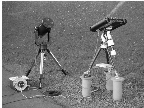
**Figure 7.** Calibration observation of the UT-DIMM (left) with the Subaru-DIMM (right) at Mauna Kea.
