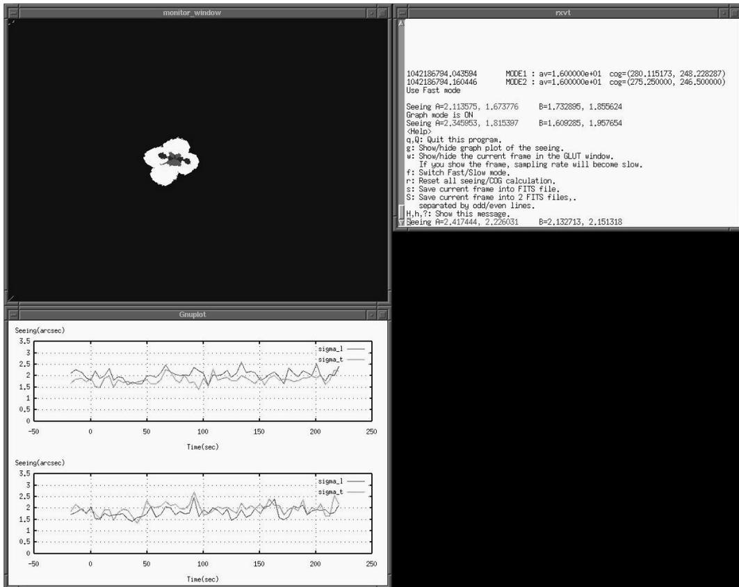
Figure 4. Screen shot of the seeing monitor software. Upper-left is a window to display captured frames and positions of COGs, lower-left is a plot of seeing, and upper-right is a console window.
