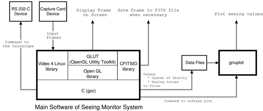
Figure 3. Block diagram of the software of the UT-DIMM.
