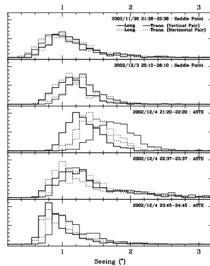
**Figure 6.** Histograms of the observed seeing during the test observations at Atacama. The solid lines show the seeing obtained from the vertical pair of the aperture, and the dotted lines from the horizontal pair. The thick and thin lines represent the data from longitudinal and transverse motions, respectively.
