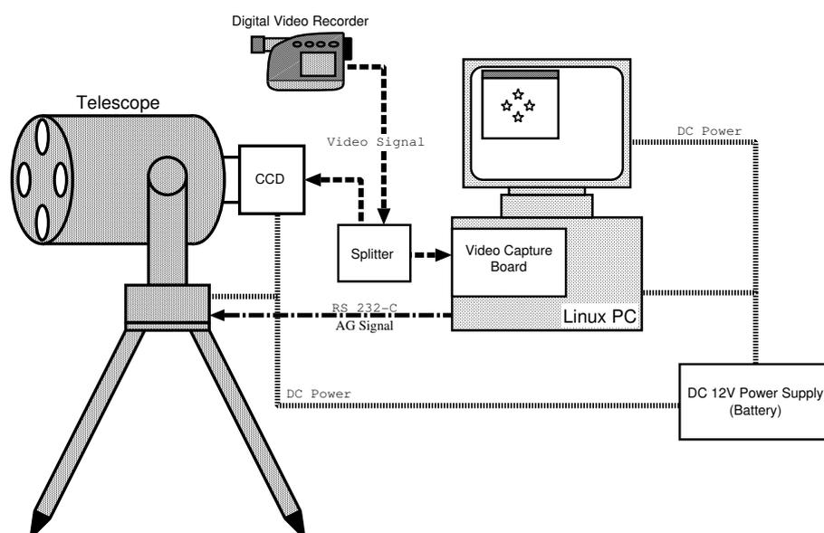
Figure 1. System overview of the UT-DIMM.
