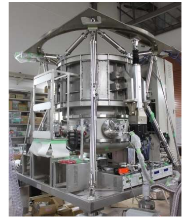
MIMIZUKU at Mitaka Lab. Dimensions are 2.0 \times 2.0 \times 2.1 m 3 . Weight is 2.5 tons.
